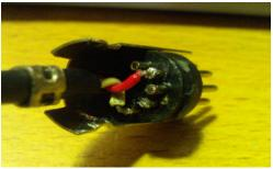
SOLDER THE WIRE TO CONNECTOR. CLAMP IT. SLIDE IN THE RUBBER COVER.
