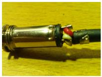
! USE MULTIMETER TO CHECK FOR THE CORRECT TAB FOR SIGNAL AND GROUND. (DIFFERENT BRAND MAY HAVE DIFFERENT LAYOUT)
