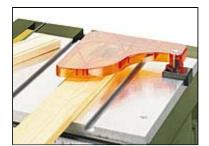
Available as an option (article-no. NO 28 736): T-slot milling device. For table saws FET and FKS/E. Consisting of milling protection and tungsten tipped saw blade 50  $\times$  2  $\times$  10mm. For cutting slots in drawers, picture frames, etc. Milling depths max. 8mm. Easy to assemble.
