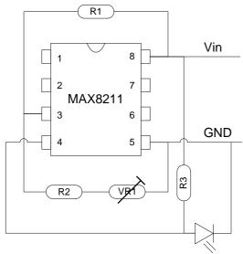
In this case the positive lead of the LED is pulled high by R3 when pin 4 is opencircuit, but when pin 4 is grounded (switched on) both sides of the LED are at the same potential and it should go off. R3 should be chosen to limit the LED current to a safe level (1K ohms perhaps).
