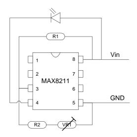
The IC is a Maxim 8211 voltage monitor designed for monitoring microprocessors. Pin 8 is the supply rail (anything from 2v to 16.5v). Pin 5 is ground.
