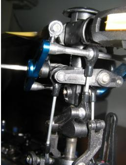
Here when it hit the blade holders. You are seeing the blade holders have been ground one side. This is because I thought by doing this way would resolve the problem. But it does not.
