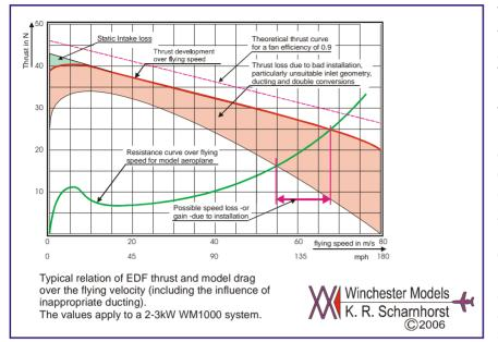
The graph on the left shows the typical thrust behaviour of a ducted fan installation. The same applies to smaller EDFs in proportion. The pink under-laid area indicates the influence of the ducting, be it very well done or rather badly; the velocity gain can be up to around 23% in this case for the same model (apart from the ducting)!
