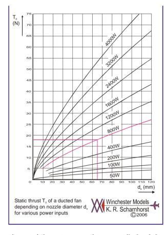
This rather basic but surprisingly accurate (and therefore useful) interrelation is depicted in the graph to the left. It shows the change of (static) thrust over the exit diameter for various powers. Alternatively for a fixed exit it shows the increase in thrust at various power levels.
